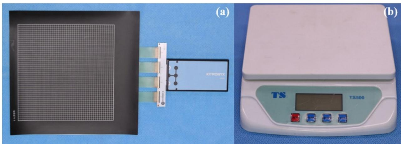
**Figure 1.** The force-sensitive resistor (MS9717) connected to data acquisition electronics (Baikal force controller) (a) and digital weighing scale (TS500) (b).
