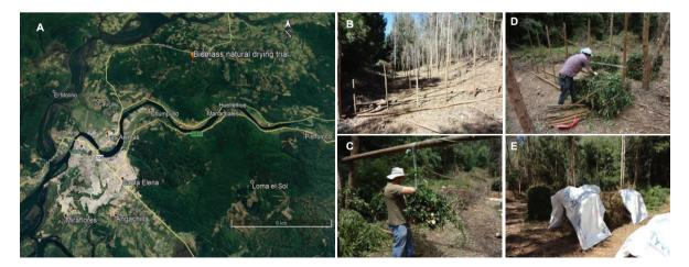
**Figure 2.** Natural biomass drying test: A) location of the study; B) delimitation of the trial with stakes; C) biomass weight; D) building of piles; E) biomass piles with and without cover.
