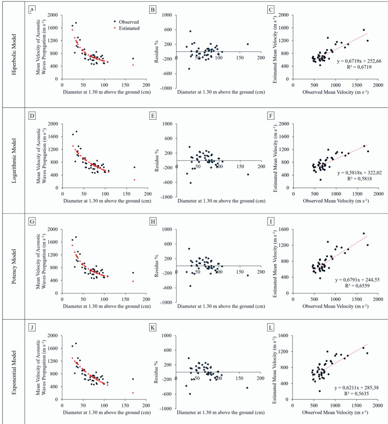
**Figure 4.** Validation graphs for the models selected to evaluate the effects of causality between the Mean Velocity of Acoustic Wave Propagation and DBH (Diameter at 1.30 m above the ground). Adjustment of models (A, D, G and J); residual distribution (B, E, H and K); validation of estimated values as a function of those observed (C, F, I and L).
