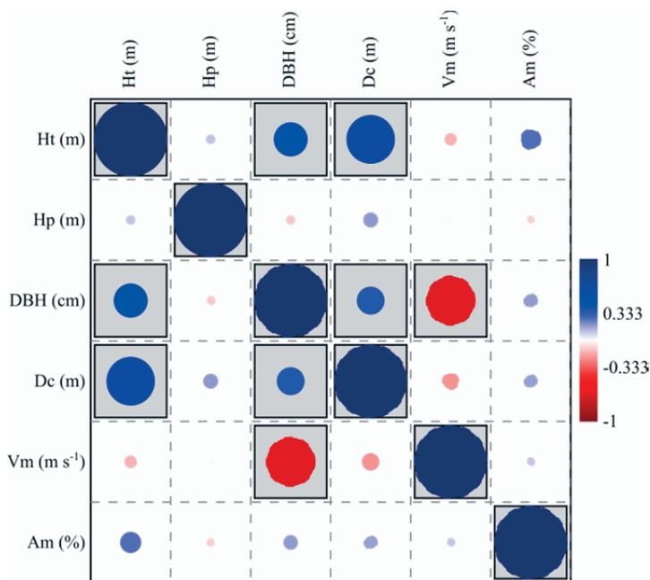
**Figure 3.** Spearman's correlation (5 % of significance) between the dendrometric variables, mean velocity of acoustic waves propagation ( $V_m$ ) and mean amplitude of perforation resistance ( $A_m$ ). The size of the circles corresponds to the strength of the correlation between variables. Significant correlations ( $P < 0.05$ ) are shown in the image. Where: Ht = total height; Hp = height to the first branch; DBH = diameter at 1.30 m above the ground; Dc = crown diameter.
