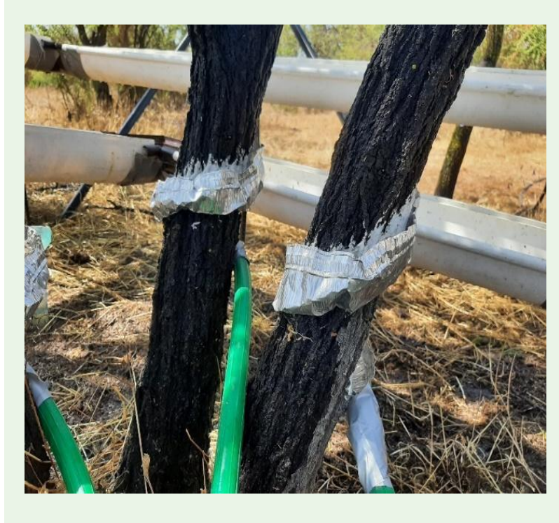
Figure 4. Detail of collars for collecting stemflow installed in V. caven .
